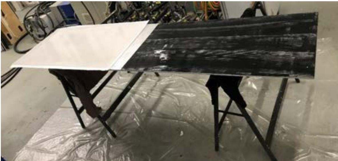
Fig.8: Silicone build up attached to one aluminium demonstrator panel
