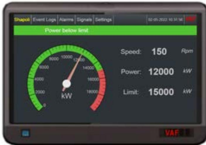
Fig.5: VAF Instruments ShaPoLi Bridge Panel PC SBP-3
