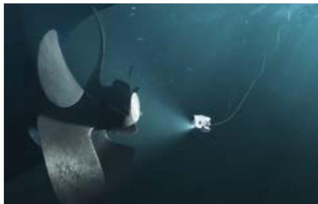
Fig.18: In-water inspection drone (Blueye Robotics)
