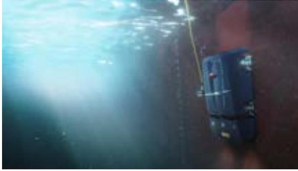
Fig.8: Hull Skater robot for proactive cleaning, [www.jotun.com](http://www.jotun.com)
