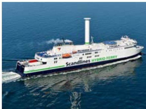
Fig.1: m/v Copenhagen with a Norsepower rotor
