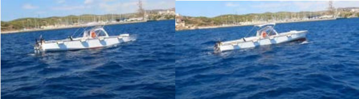
Fig.12: Instances of tests of NTUA large-scale model in wave conditions at sea, without the foil
