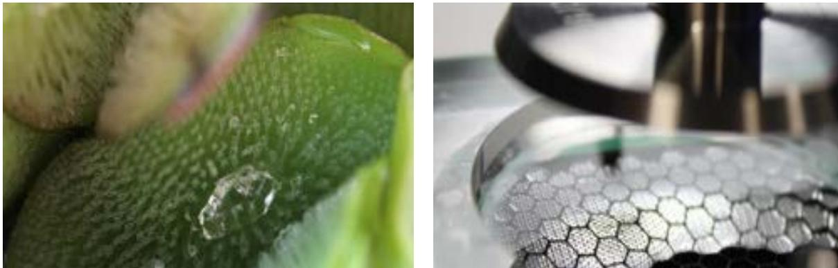
Fig.6: Floating fern (left) inspired the passive air-trapping foil (right) in the AIRCOAT project
