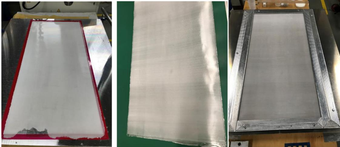
Fig.7: left: casting of the reinforced silicone film; middle: free silicone dermis; right: frame set up on the silicone dermis, ready to be filled up with blubber material
