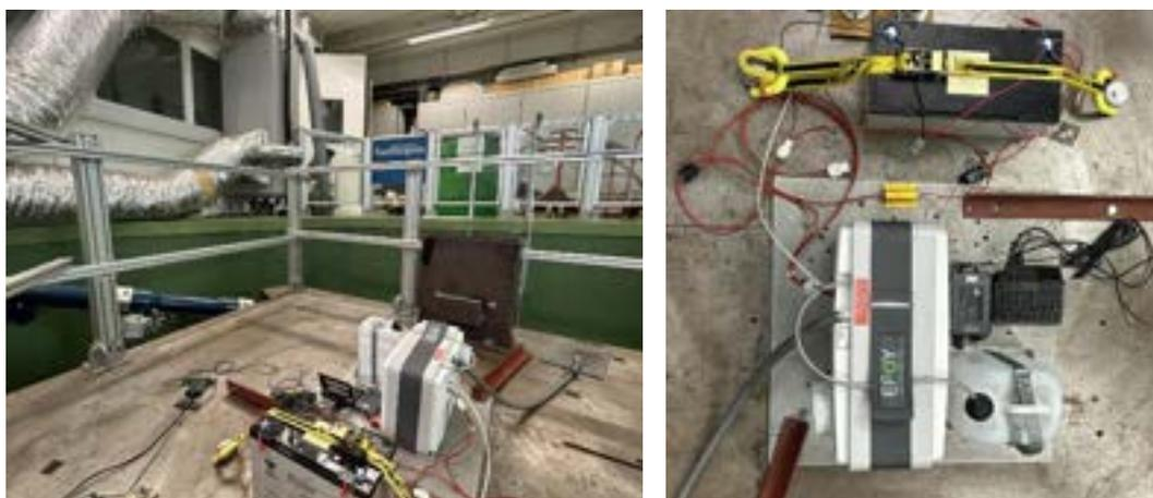
Fig.1: View of fuel fell experiment Set-Up of Shaker (Left) and equipment (Right)
