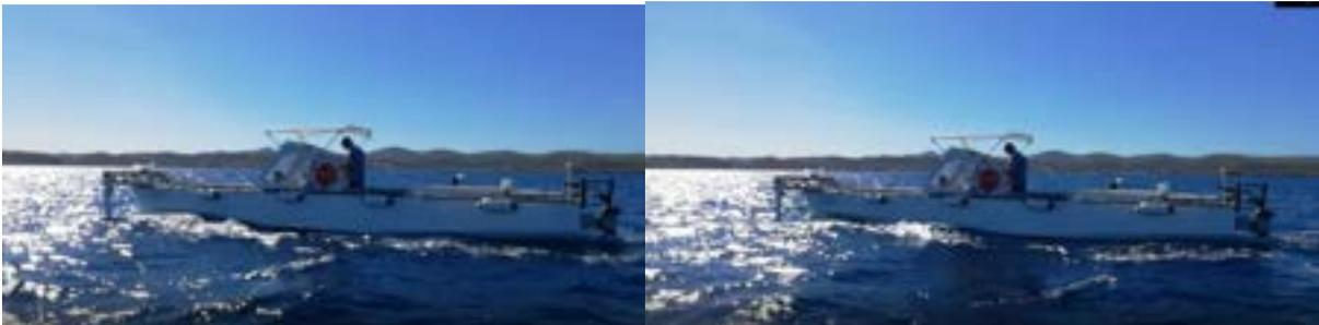
Fig.13: Instances of tests of NTUA large-scale model in wave conditions at sea, with the operation of the dynamic foil at the bow
