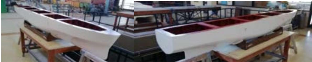
Fig.1: NTUA tank-scale hull model of  $L/B = 7.67$  used for tests
