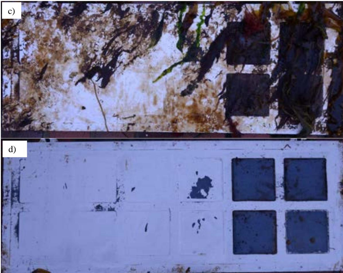
Fig.6: Static immersion testing of compliant coatings. a) panel before static immersion, b) after 5 months (October 2022), c) after 11 months (March 2023) when the experiment was terminated by assessing the ease of biofouling removal: d) cleaned panel
