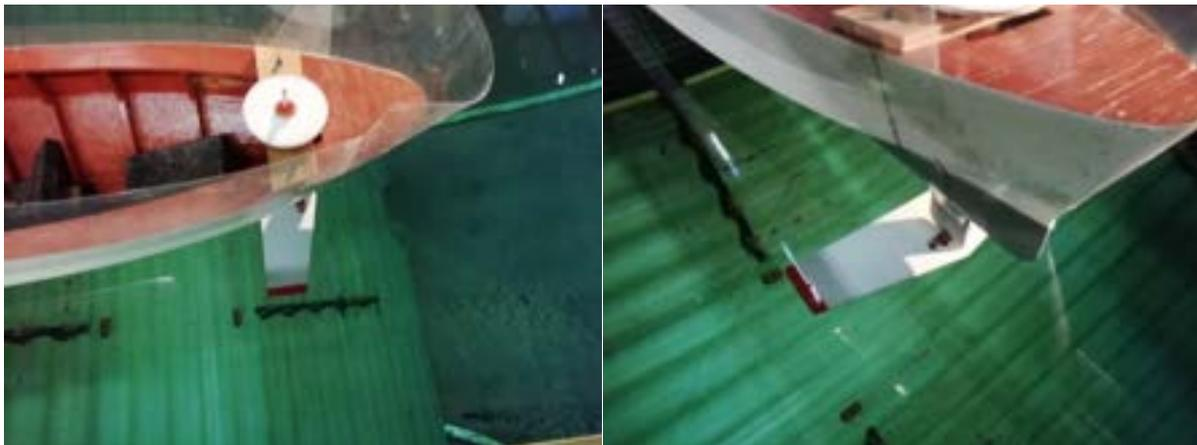
Fig.19: Tank tests of the NTUA ferry ship model with a T-foil at the bow in calm water
