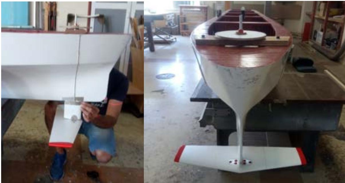
Fig.18: The NTUA ferry ship model with a T-foil arrangement at the bow
