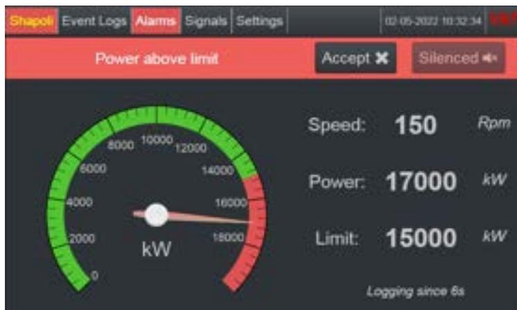
Fig.6: SBP-3, power exceeding EEXI limit alarm screen
