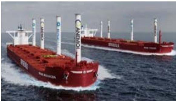
Fig.11: Tiltable Flettner rotors on bulk carriers, source: Berge Bulk
