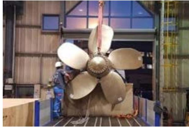
Fig.20: 3D printed propeller, source: Naval Group
