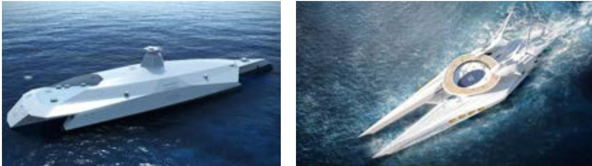
Fig.2: Multihull design concept for future warship (left) and cruise vessel (right)
