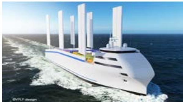
Fig.12: Vision of cargo ship with many rigid sails, source: <https://www.vplp.fr/en/shipping/>
