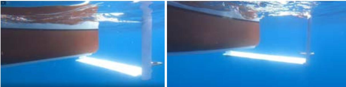
Fig.14: Underwater shots of the dynamic wing operating at the bow of the large NTUA ship model
