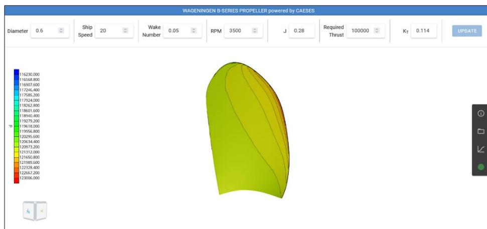
Fig.10: Screenshot of the New Wageningen Web Application – Pressure Distribution Displayed
