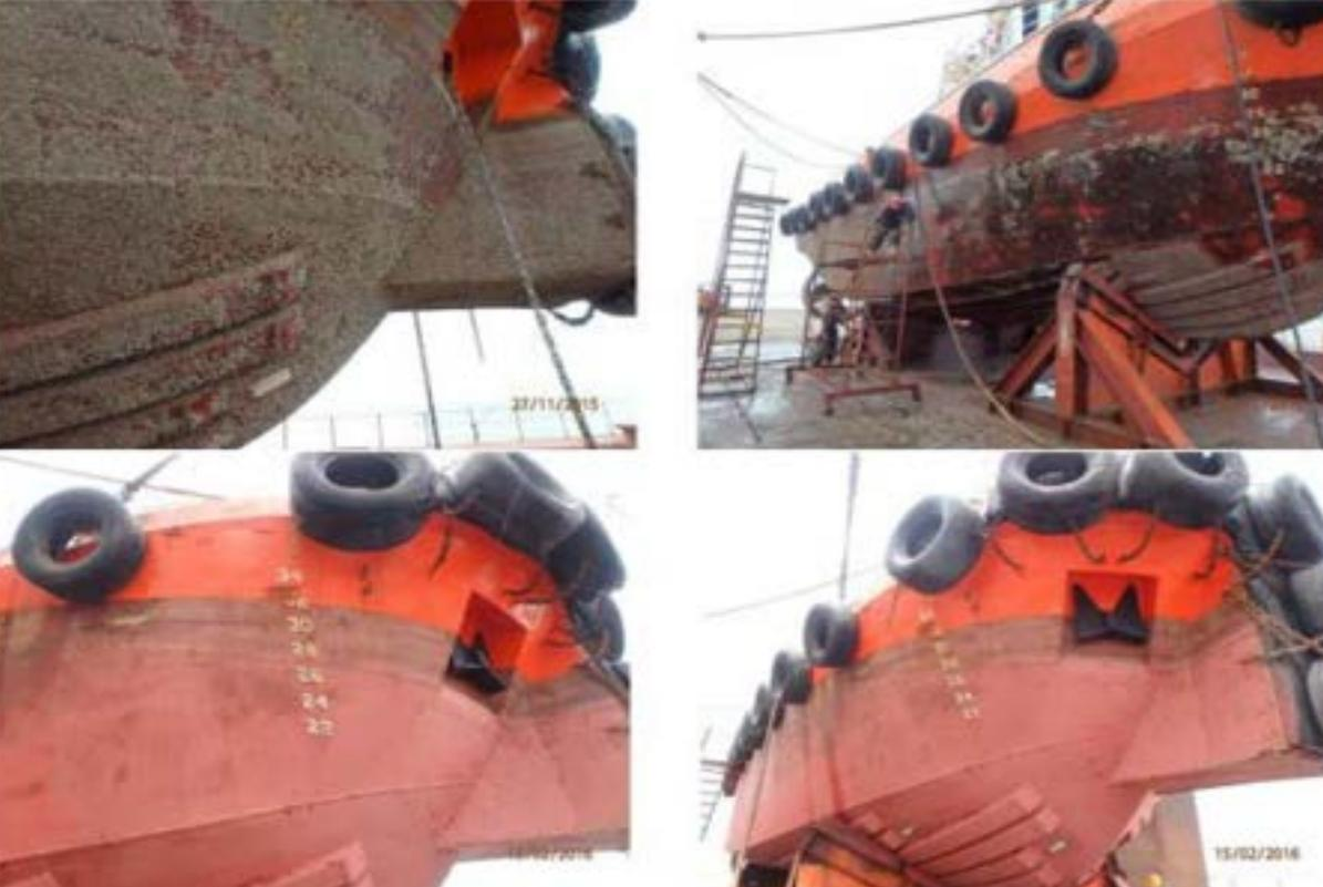
Fig.7: Tugboat without (top) and with (bottom) ultrasonic antifouling protection
