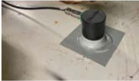
Fig.7: Application of coating after transducer gluing (example from sea chest installation)
