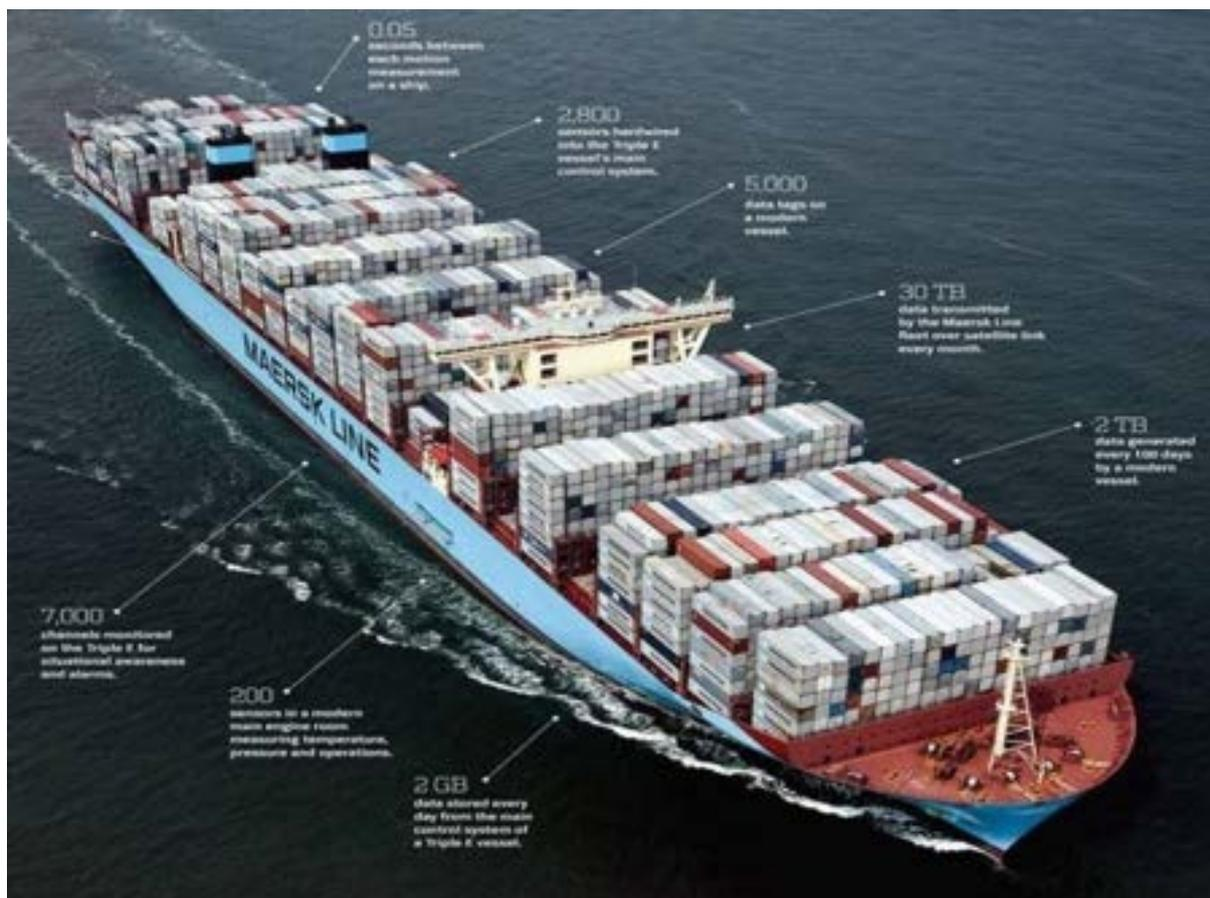
Fig13: Modern ship with extensive sensor network (2017), source: Maersk
