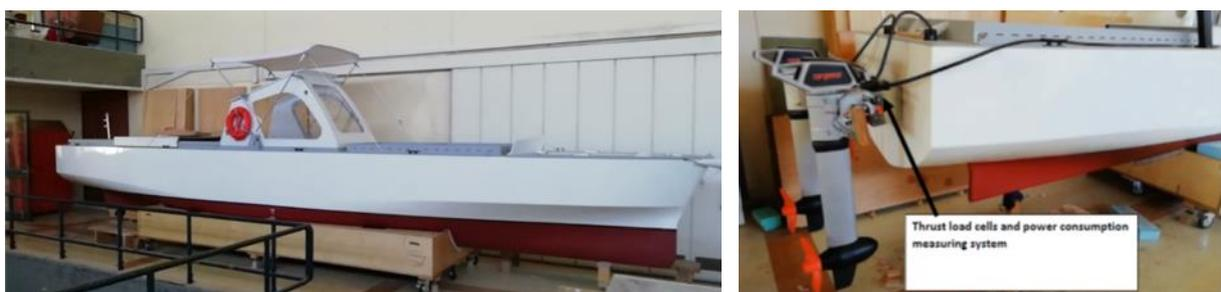
Fig.9: Completed NTUA large model of length 10 m and standard propulsion system at the stern using electric outboard engines for standard propulsion of the large-scale model
