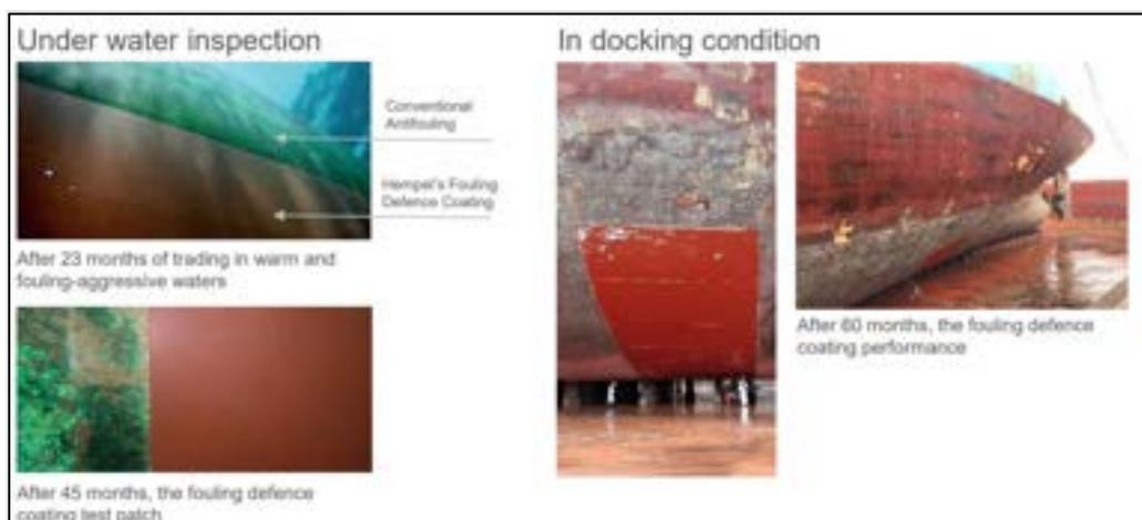
Fig.1: The surface condition of a ship hull coated with/without Hempaguard
