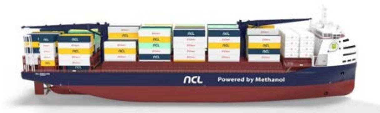
Fig.5: Prototype of future feeder ship using Methanol as fuel, source: NCL (2022)
