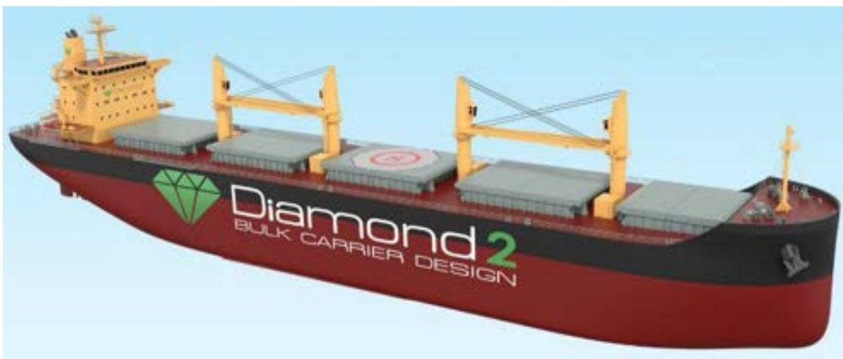
Fig.3: Diamond 2 bulk carrier design with straight stem at bow
