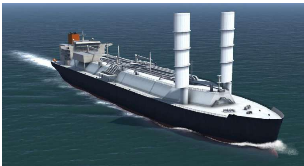
Fig.18: Installation example for LNGC (2 sails)
