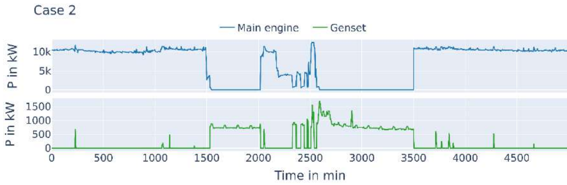
Fig.11: Operating profiles for the Case 2 configuration: Main engine, genset, shaft generator
