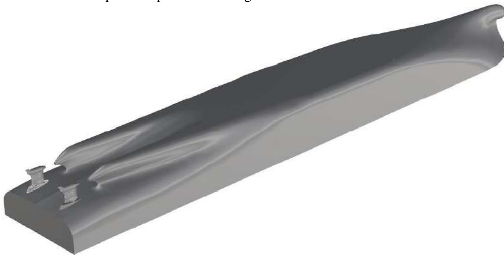
Fig.1: 3D model of the final hull version of the ULCS with the twin-CRP-pod propulsion system
