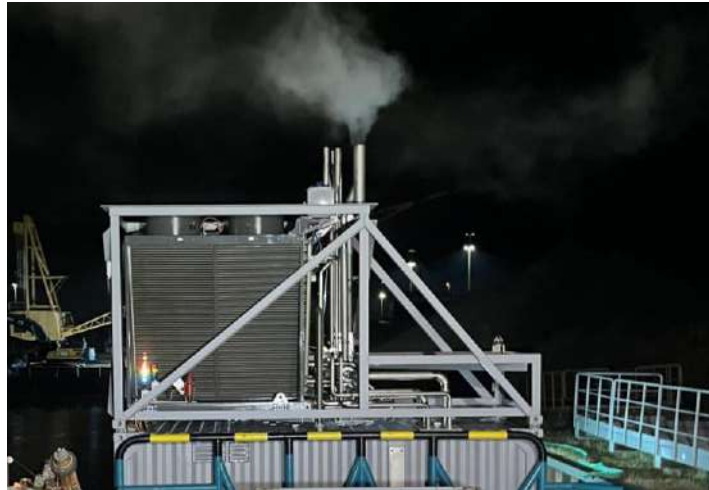
Fig.7: V-shaped cooler and vent masts on top of the eCap H2 PowerPac
