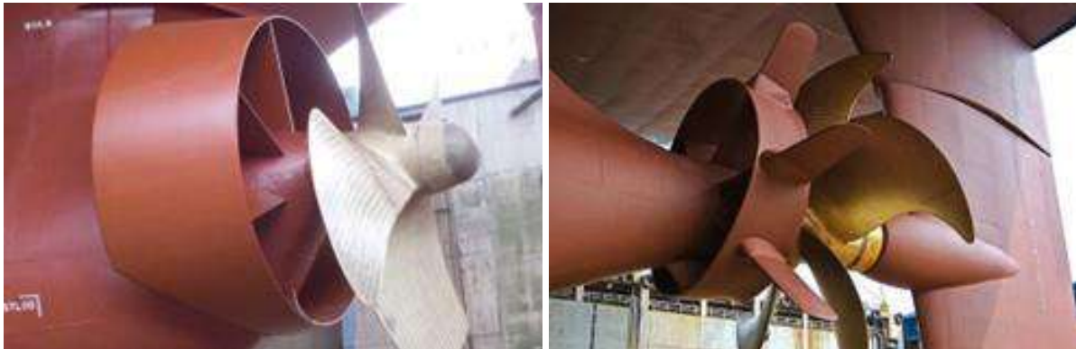
Fig.3: Becker Mewis Duct® (left) and Becker Twisted Fins® (right) after installation at the shipyard
