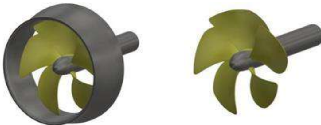
Fig.3: Propeller with (left) and without (right) duct
