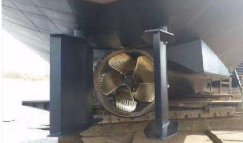
Fig.4: Final propeller mounted on the ship; the duct is part of the hull
