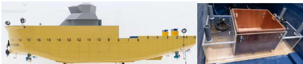
Fig.17 - Seakeeping model as tested at MARIN, along with the U-type ART
