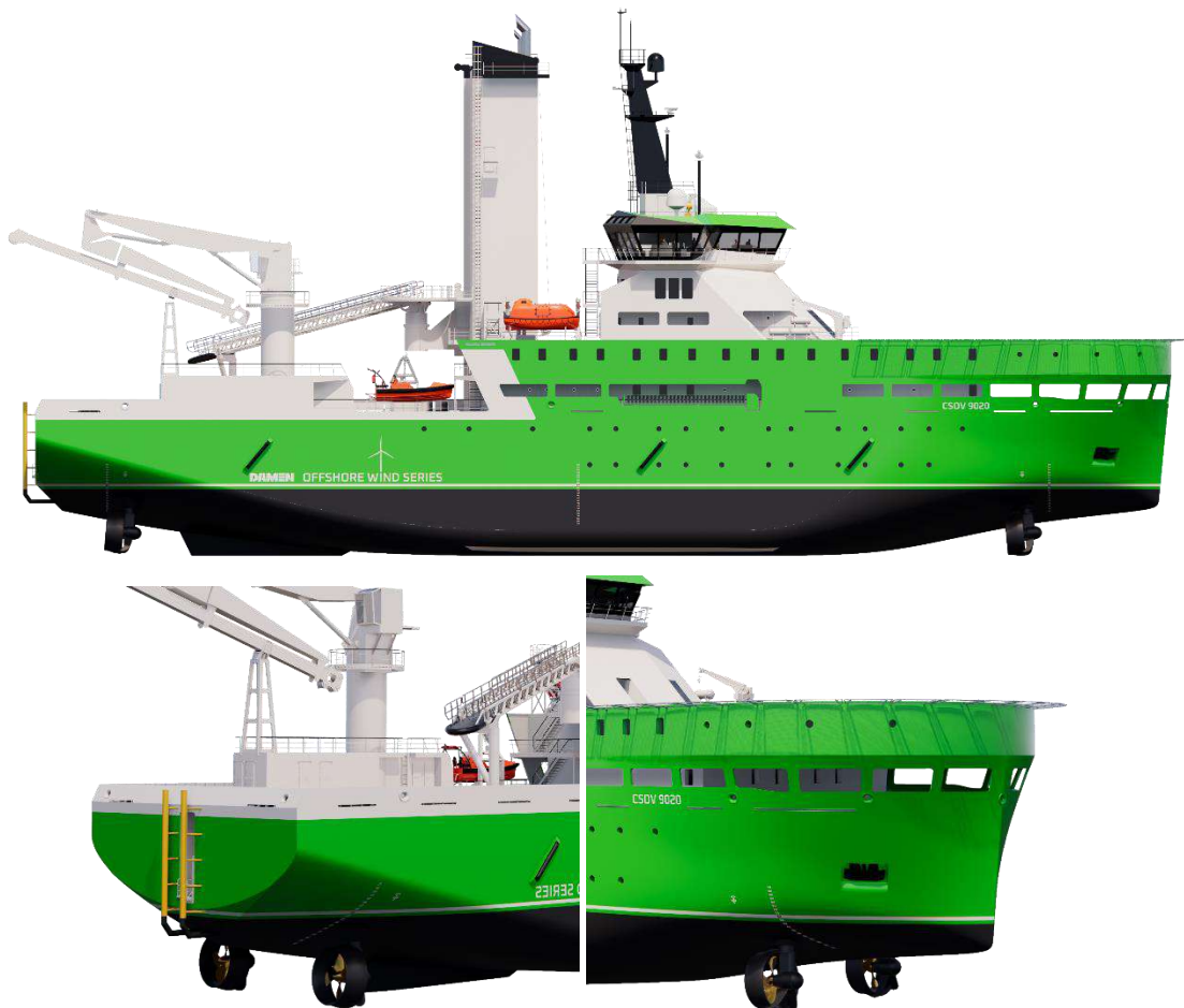
Fig.3: Hull shape of the new CSOV Design showing the forward and aft ends of the vessel. ©Damen Shipyards Group
