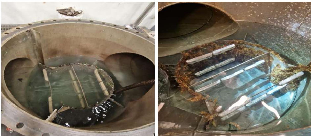
Fig.6: Results from test voyage trials – Sea strainer after 1 year; with (left) and without (right) ultrasonic protections
