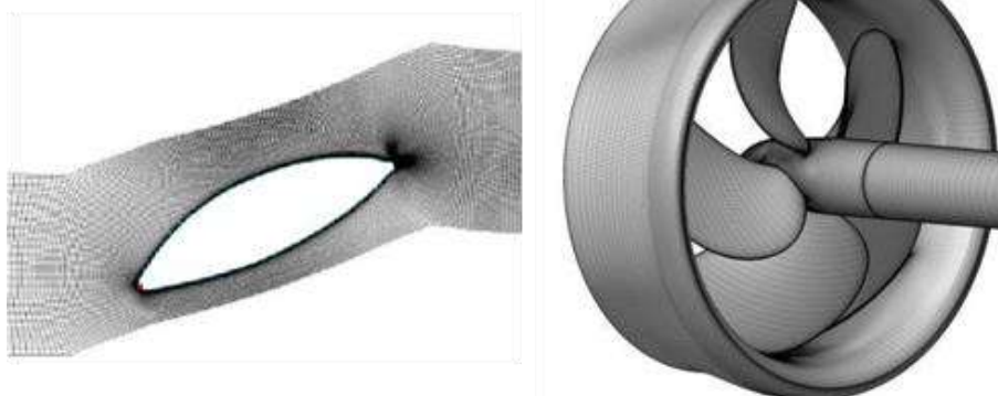
Fig.7: Final mesh: blade-to-blade view at 0.2R (left) and mesh repetition (right)
