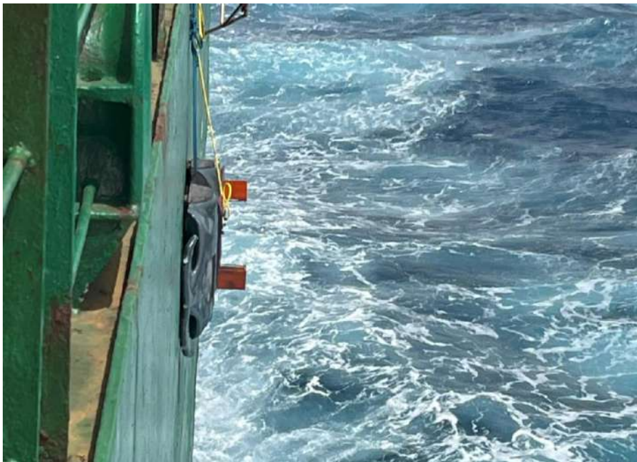
Fig.3: NakAI's Goby robot during one of the in-transit sea trials. The foils, which assist in generating additional downforce and are seen in red, are set to an open state.
