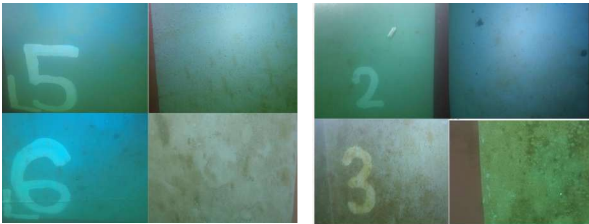
Fig.9: Hull text patches, with (top) and without (bottom) ultrasonic protection
