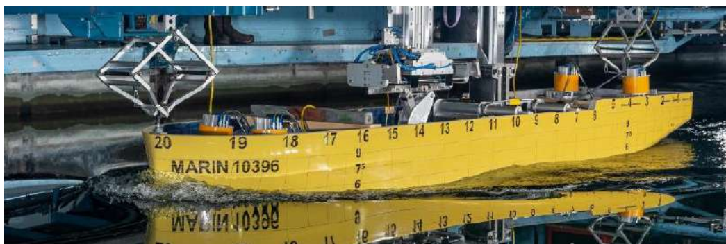
Fig.11 – Self-propulsion model tests as performed at MARIN's towing tank (14kn)
