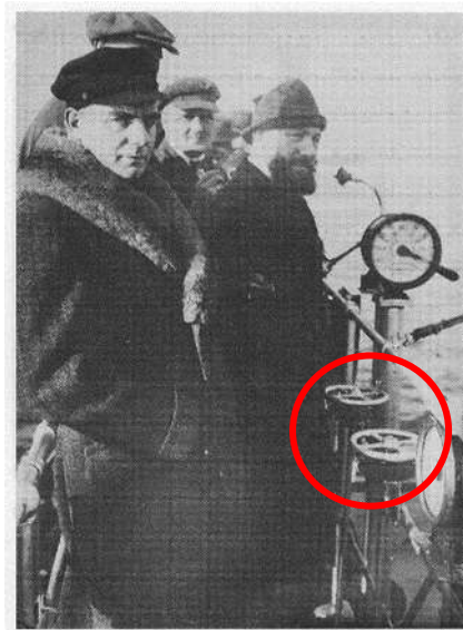
Fig.9: Controls on BUCKAU - 2 handwheels, Flettner (1926)
