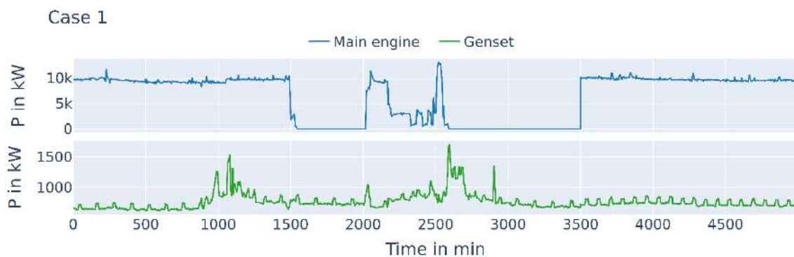
Fig.10: Operating profiles for the Case 1 configuration: Main engine, auxiliary genset
