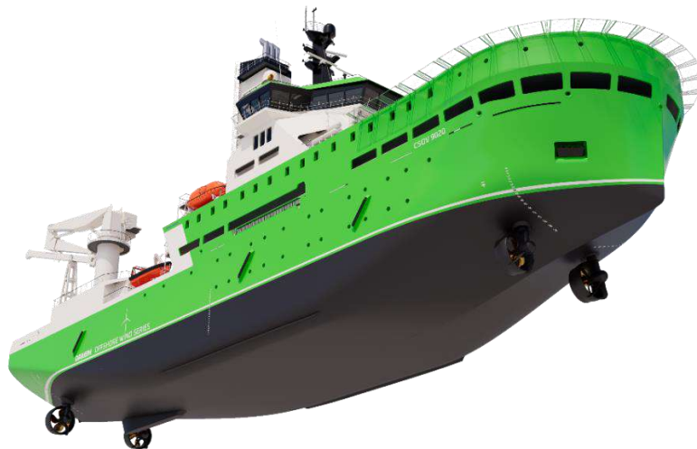
Fig.2: Damen DPX™ Drive with 4 identical thrusters installed on the CSOV9020. ©Damen Shipyards Group
