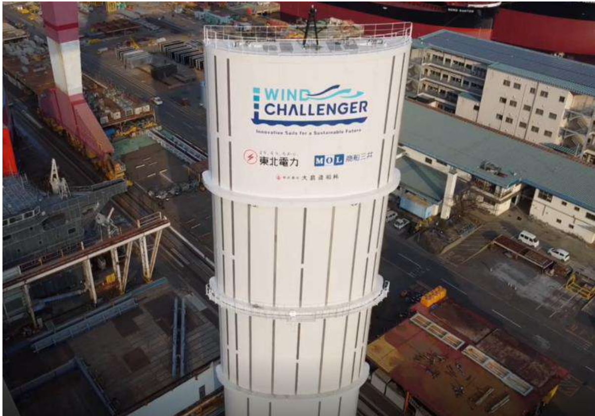
Fig.2: The hard wing sail named Wind Challenger has been developed by MOL
