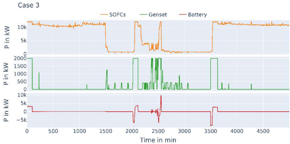
Fig.12: Operating profiles for the Case 3 configuration: SOFCs, genset, battery
