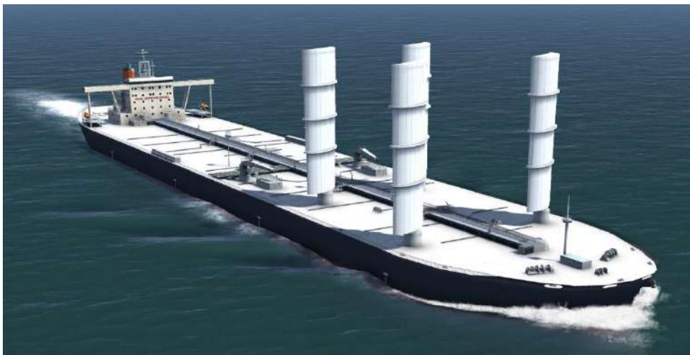
Fig.17: Installation example for VLCC (4 sails)
